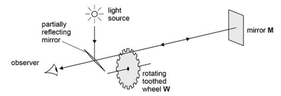
The toothed wheel  ${\bf W}$  is rotated and the reflected light from a distant mirror  ${\bf M}$  is observed.
